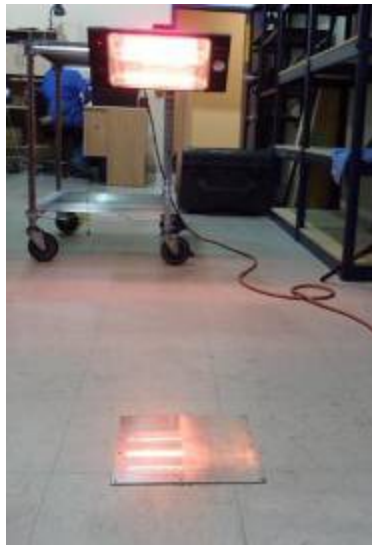
Figure 12. Test configuration with quartz lamp and Al target.
